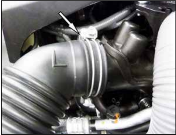
4. Loosen the hose clamps that secure the factory upper intake tubes to the turbo inlet manifolds and then remove the upper housings, intake tubes and filters. NOTE: K&N Engineering, Inc., recommends that customers do not discard factory air intake.
