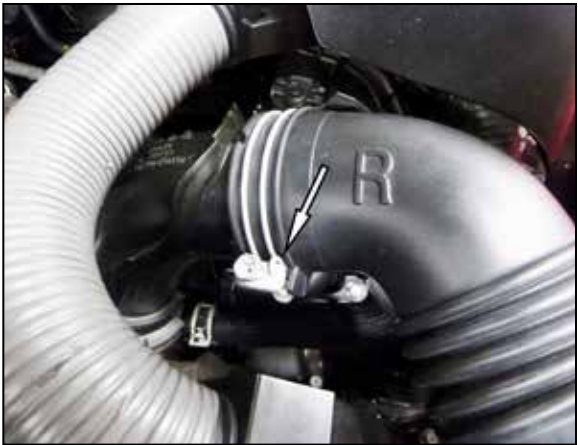
3. Release the retaining clips that secure the upper air filter housings.
