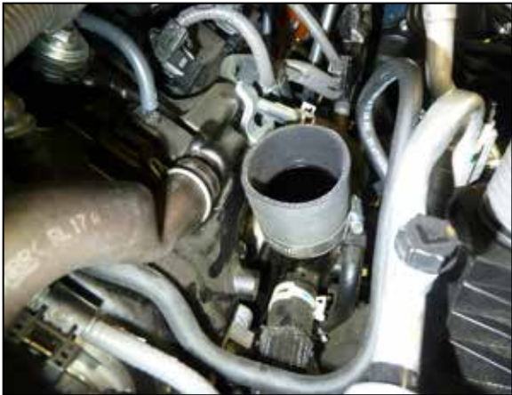
9. Install the provided couplers onto the turbo inlets and secure with the provided hose clamps.
