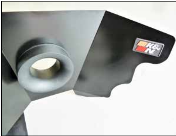
9. Install the provided couplers onto the turbo inlets and secure with the provided hose clamps.
