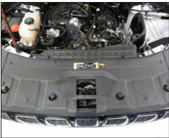
14. Reinstall the radiator cover and secure with the factory mounting pins.
