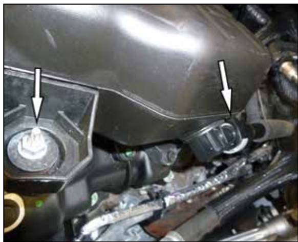
4. Remove the nut that secures the intake tube to the mounting bracket and then disconnect the CCV hose connector. Remove the intake tube from vehicle.
