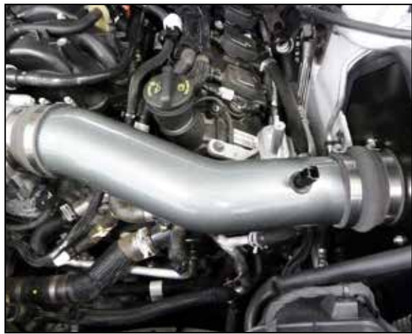
20. Install the intake tube into the couplers, adjust for best fit and then secure with the hose clamps.
