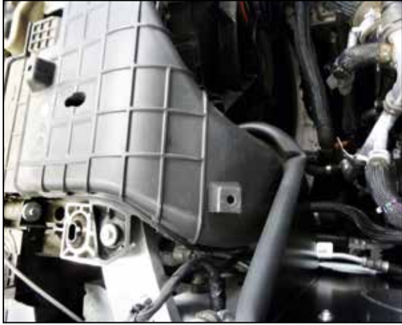
13. Reinstall the fresh air intake duct and align with the heatshield.
