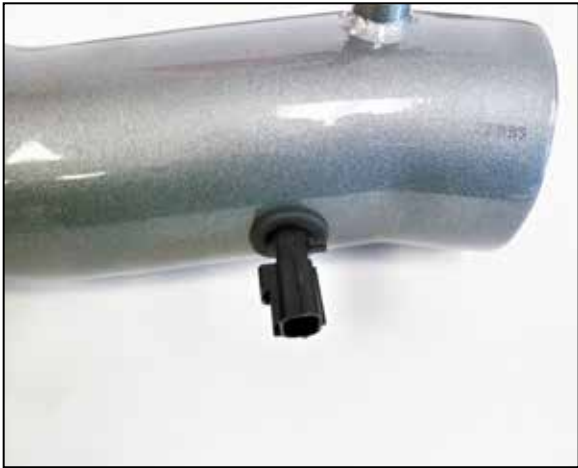
16. Install the IAT sensor into the K&N intake tube using the grommet provided.
