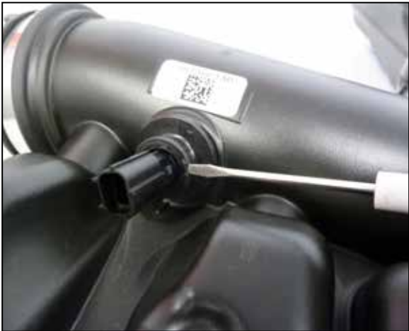
15. Release the locking tab on the IAT sensor and then rotate and remove the sensor from the factory intake tube.
