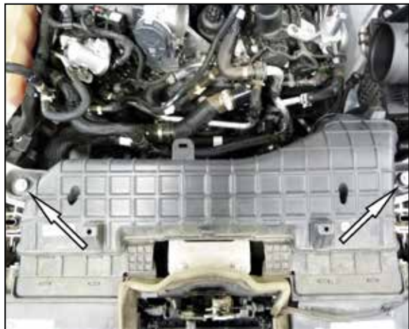
6. Remove the two bolts that secure the fresh air duct and then remove the duct from the vehicle.
