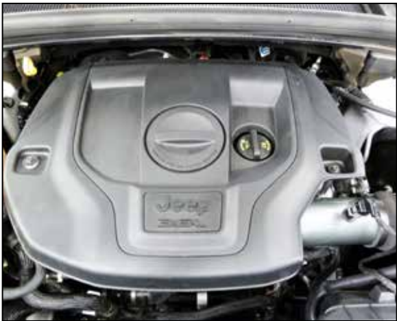
24. Reinstall the engine cover and secure with the factory hardware.
