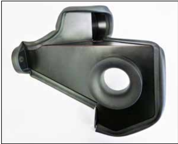
11. Install the edge trim around the heatshield as shown. NOTE: some trimming of the edge trim will be necessary.
