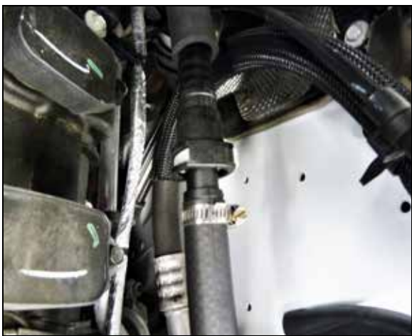
21. Connect the CCV extension to the factory CCV quick connect.
