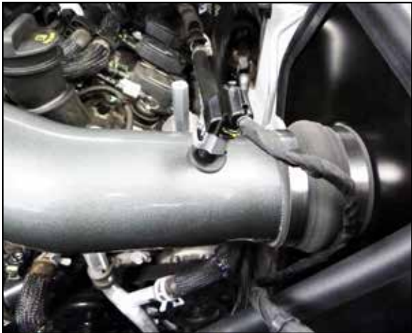
22. Reconnect the IAT sensor electrical connection.
