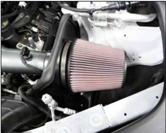
23. Install the air filter onto the filter adapter and secure with the provided hose clamp.
