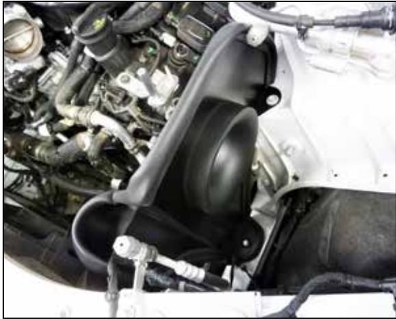
12. Install the heatshield into the vehicle so the mounting grommet engages the mounting stud and then secure the heatshield with one of the factory air filter housing mounting bolts.
