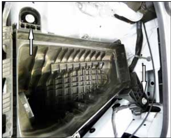
8. Remove the two bolts that secure the lower air filter housing and then remove the housing from the vehicle. NOTE: K&N Engineering, Inc., recommends that customers do not discard factory air intake.
