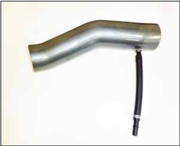
18. Install the CCV extension into the K&N intake tube as shown. NOTE: The fitting threaded into the tube is 1/4"npt, do not over tighten.
