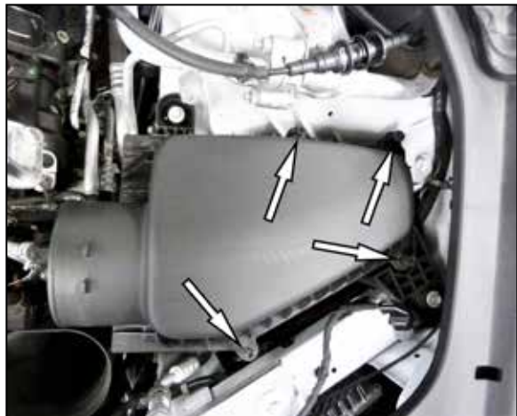
7. Loosen the four bolts that secure the upper air filter housing, remove the upper housing and factory air filter.
