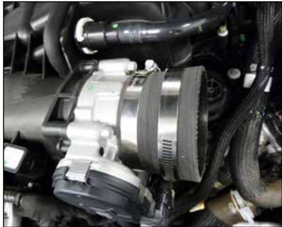
19. Install the provided couplers and secure with the provided hose clamps, The hump coupler goes onto the filter adapter and the straight coupler attaches to the throttle body.
