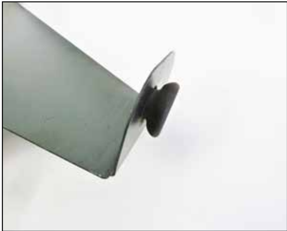
10. Remove one of the mounting grommets from the factory lower air filter housing and install it into the heatshield.
