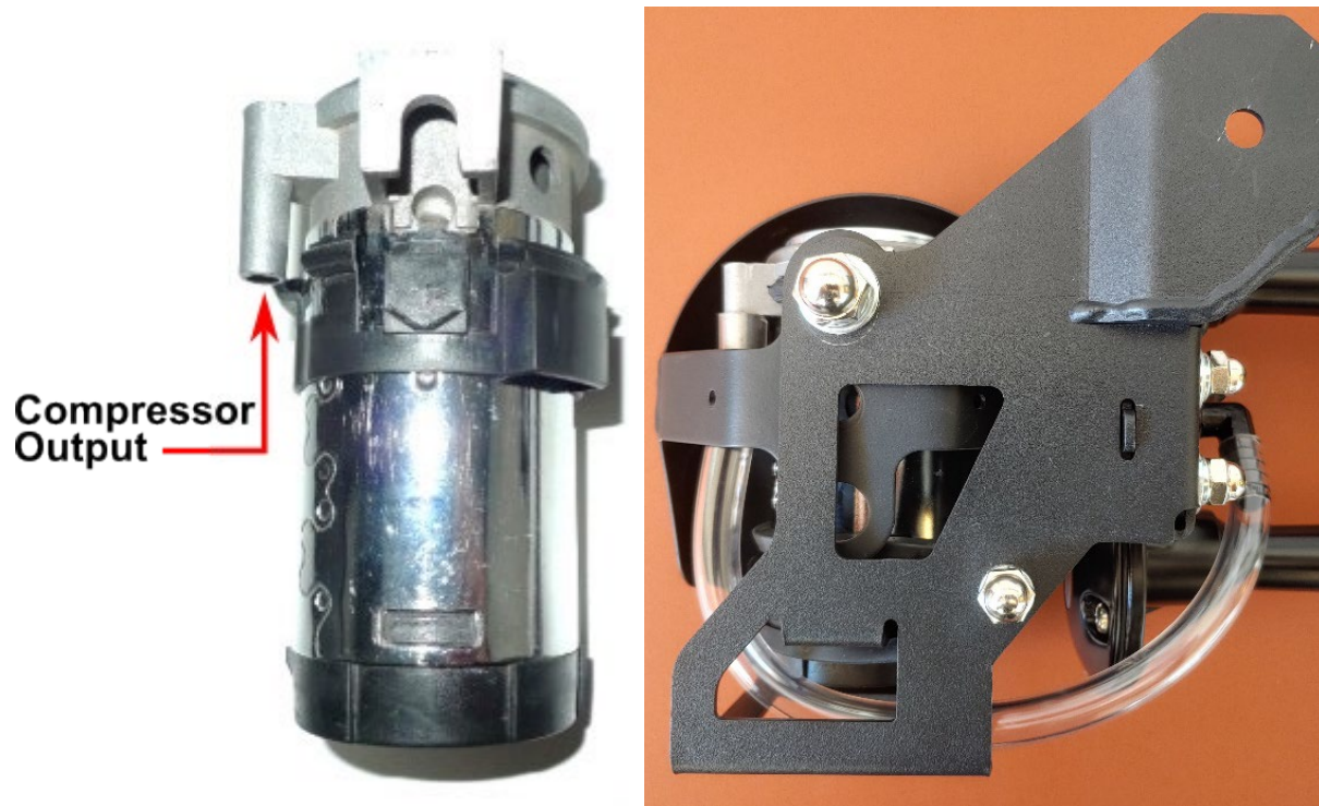
Figure 18- Plumbing Compressor to Horn
