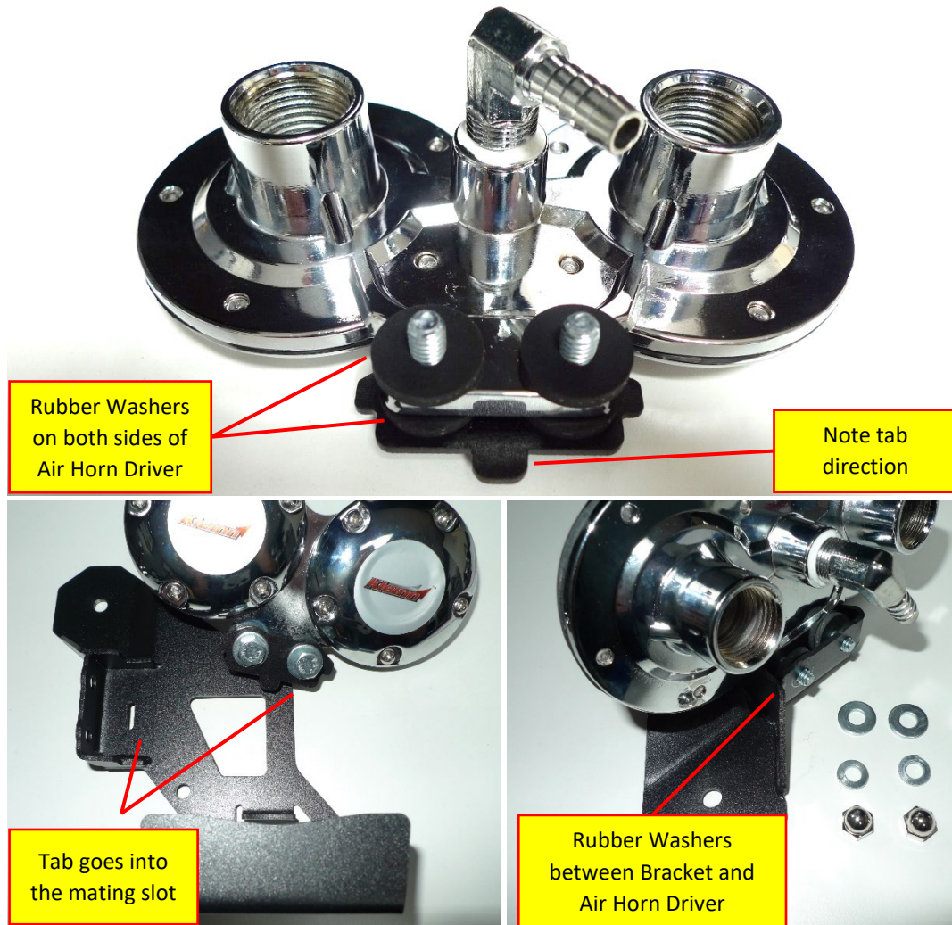
Figure 9- Horn Driver Install
