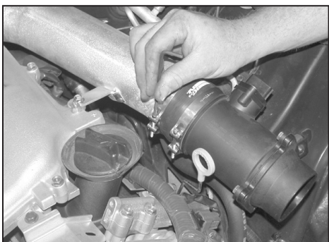
16. Slide the mass air sensor assembly onto the intake tube and tighten the hose clamp.
