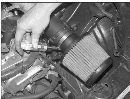
17. Install the K&N® air filter and secure with the provided hose clamp as shown. NOTE: Drycharger® air filter wrap; part # RX-4990DK is available to purchase separately. To learn more about Drycharger® filter wraps or look up color availability please visit http://www.knfilters.com ®.
