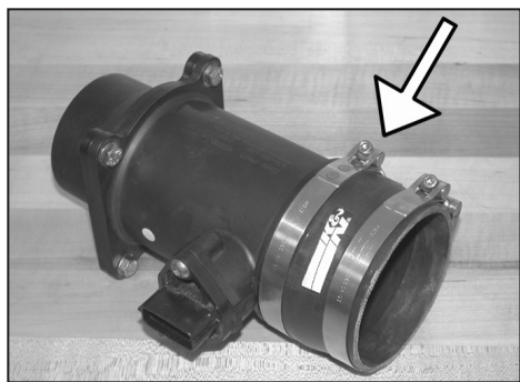
15. Install the silicone hose and hose clamps onto the mass air sensor and tighten.
