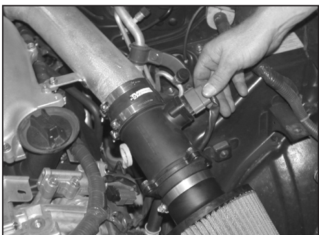
19. Reconnect the mass air sensor electrical connection as shown.
