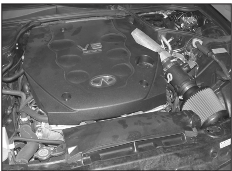
21. Reconnect the vehicle's negative battery cable. Double check to make sure everything is tight and properly positioned before starting the vehicle.
