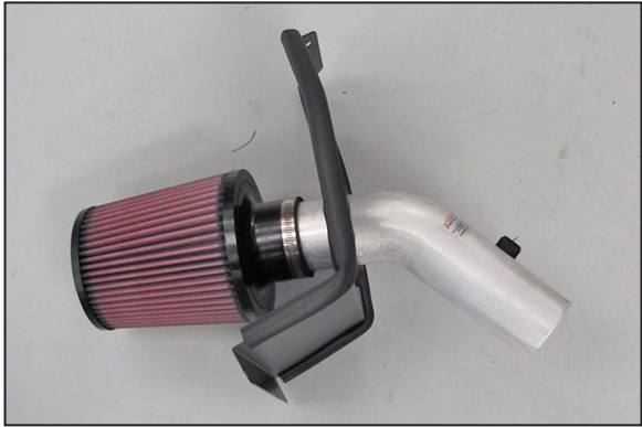
15. Install the K&N® intake tube through the heat shield as shown and then install the K&N® air filter onto the intake tube and secure with the provided hose clamp.
