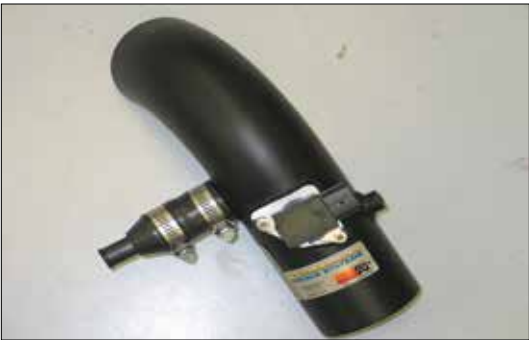
29. Install the stock mass air sensor into the intake tube and secure with the provided hardware.
