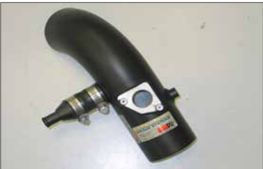
27. Install the stock crank case vent chamber into the silicone hose installed onto the intake tube secure with the provided hose clamp.
