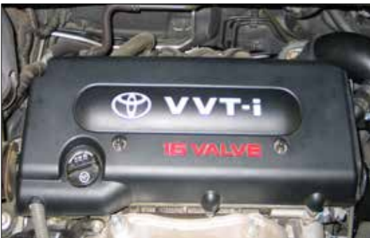
33. Install the stock engine cover and secure with the stock mounting bolts removed in step #10.
