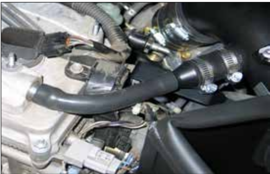
32. Install the provided crank case vent hose onto the crank case vent chamber and valve cover fitting.
