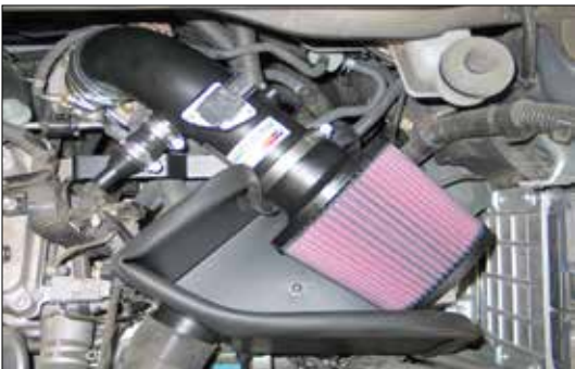
31. Install the intake tube assembly into the silicone hose installed onto the throttle body. Align with the intake tube mounting bracket installed in step # 16; then, secure the intake tube assembly using the provided hose clamp and hardware.
