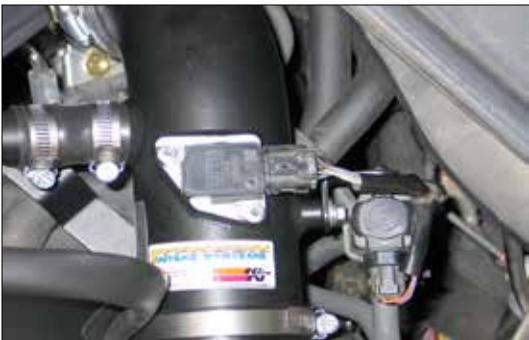
35. Re-connect the mass air sensor electrical connection.
