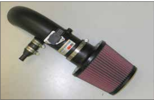
30. Install the air filter onto the intake tube secure using the provided hose clamp.
