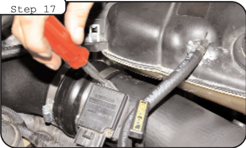
Remove mass sensor and filter minder gasket from factory housing. Install sensor onto tube using gasket, spacers and screws supplied. Install filter minder onto tube. Use factory rubber grommet.
