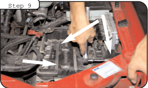
Using a 13mm socket or wrench Remove all screws holding the battery tray in the vehicle.
