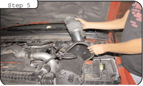
Undo the two retaining clips securing the air box outlet. Lift up and remove the turbo inlet tube and filter lid as one piece.
