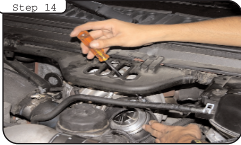
Install grey high temp silicon coupling onto turbo. Tighten clamp at turbo.
