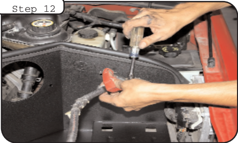
Install rubber grommet onto housing. With both batteries disconnected remove wire from terminal using a 10mm socket and pull wire through housing and reconnect.
