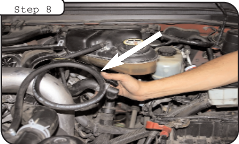
Using a 10mm socket or wrench remove tube support bracket from engine. Loosen clamp at turbo with a 5/16 nut driver or screwdriver.
