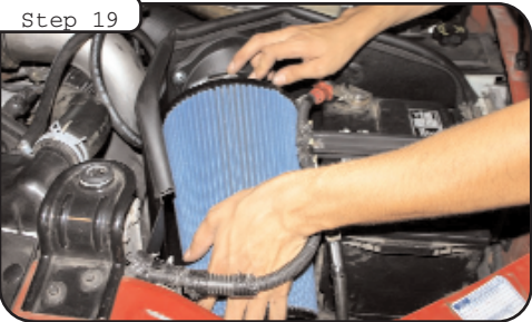
Install filter onto tube. Tighten clamp.
