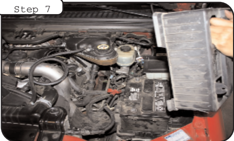
Disconnect passenger side battery terminals, remove battery cover and battery from engine compartment.
