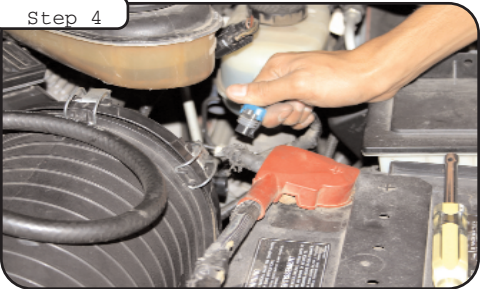
Disconnect the Filter Minder located on the back of the air filter box.
