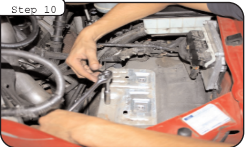
Remove battery tray support bracket from vehicle using a 13mm socket or wrench.
