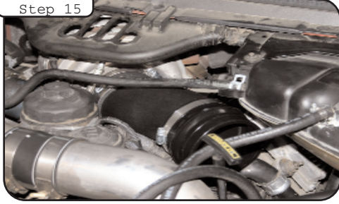
Slide tube onto coupler and reconnect crank case breather. Install hump coupler onto end of tube.
